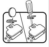
4. Replace the battery cover and tighten the screw to secure.
